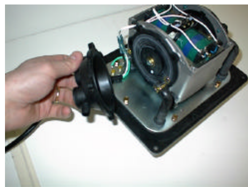
H. Remove the valve box (12).
