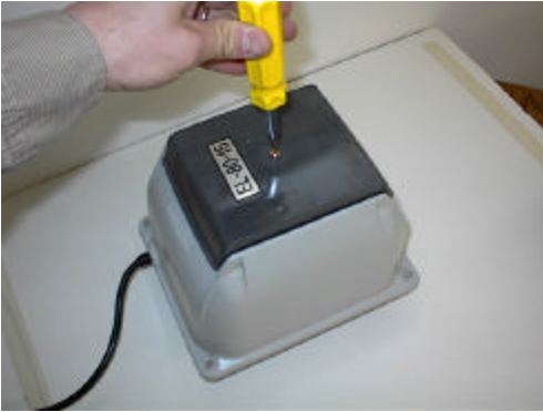
A. Remove screw (31) from the filter cover.
