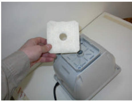
C. Shake out dust from the filter element (2). If the filter element is heavily soiled, then wash in mild soapy water and let it dry completely. Replace the filter if it has deteriorated.
