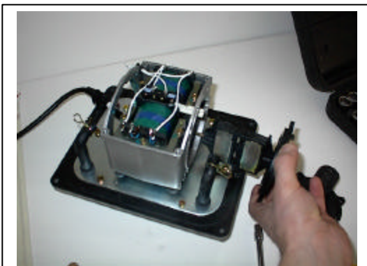
B. Remove the diaphragm holder (10) and the magnet (9) after opposite diaphragm holder (10) has been removed.
