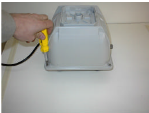
A. Remove the 4 exterior bolts (27)
